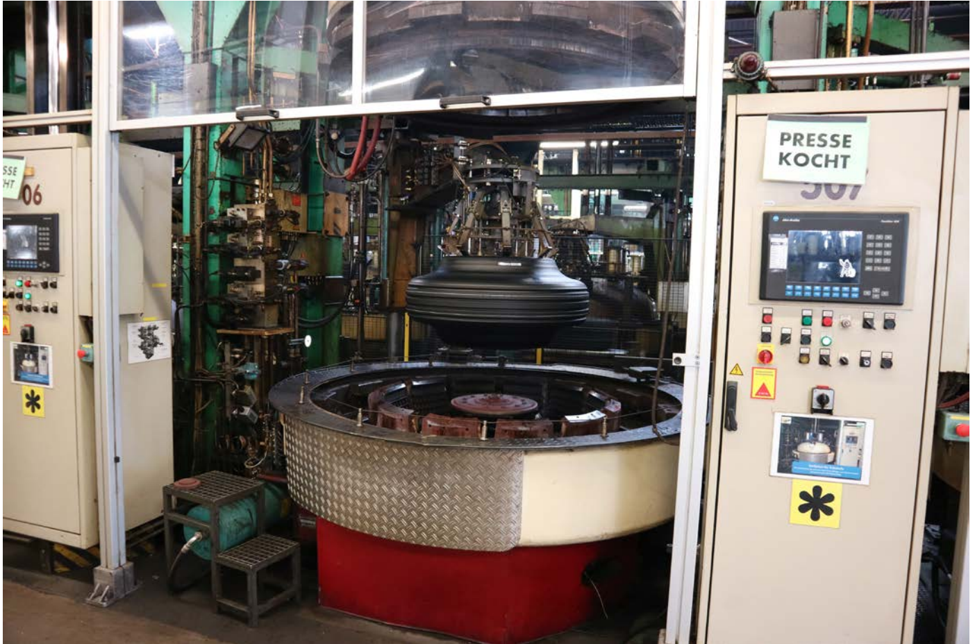
In the tire-cooking, the liquid rubber is inserted from the above into the vulcanization press, then the mold is closed with a lid and the tire brought under pressure and temperature in the final form and consistency.
