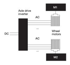
Example of an axle power efficiency measurement from DC (7) to dual 3-phase AC (1 to 3 and 4 to 6) plus dual mechanical power (M1 and M2)  $\,$
