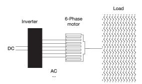
Example of an axle power efficiency measurement from DC (7) to dual 3-phase AC (1 to 3 and 4 to 6) plus dual mechanical power (M1 and M2)  $\,$
