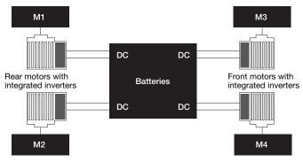
Modern drive systems with integrated inverters do not allow access to the AC signals. Here one of the main measurement tasks is the overall drive train efficiency from DC to mechanical power. The example shows 4 DC measurements (1 to 4) with the corresponding 4 mechanical power measurements (M1 to M4)
