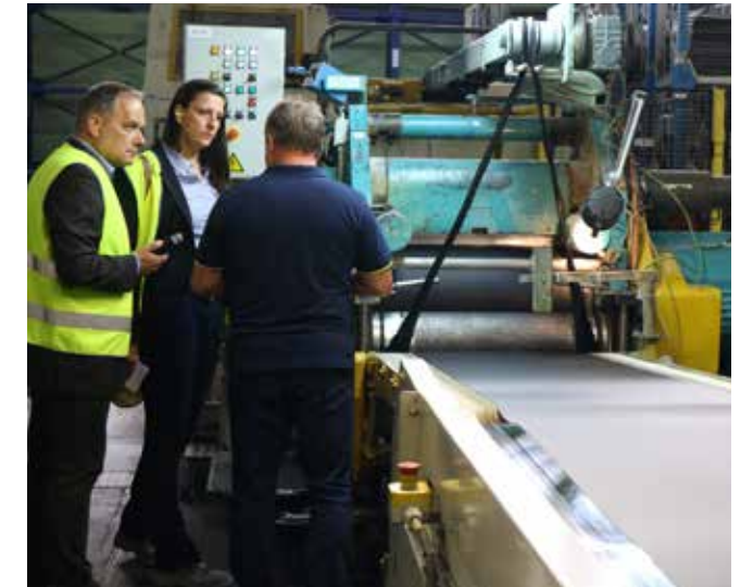
This plant produces with an extruder the inner rubber layer for truck tires. The rubber band is wound up after short cooling on large rolls and later cut to the required size.
