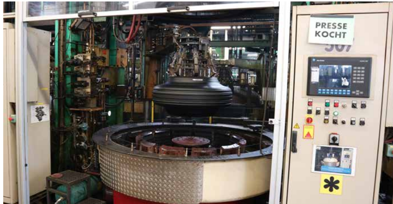
In the tire-cooking, the liquid rubber is inserted from the above into the vulcanization press, then the mold is closed with a lid and the tire brought under pressure and temperature in the final form and consistency.
