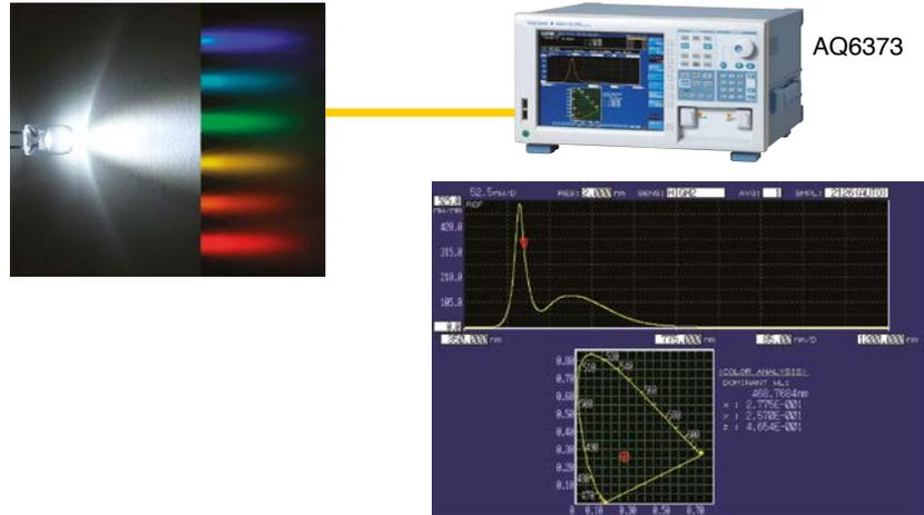
Figure 2 - Analysis of V2V LED communications with Yokogawa AQ6373B Optical Spectrum Analyser
