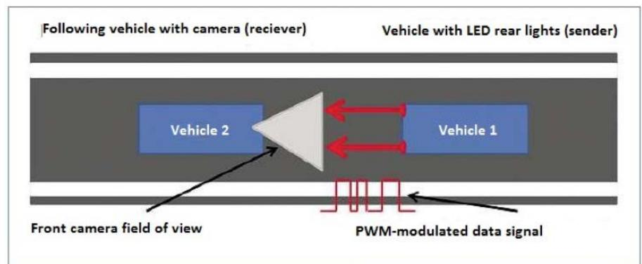
Figure 1: The main LED V2V communications system components shown as a block diagram
