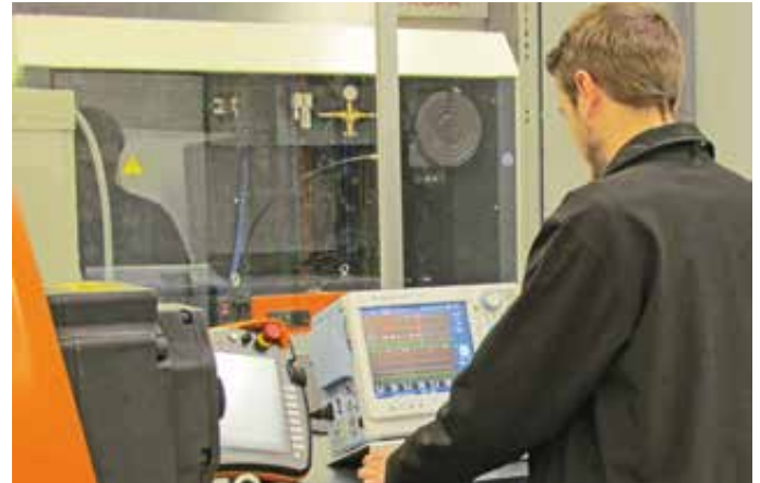
Tobias Zimmermann (KUKA Systems) measures the power consumption of the robot with the Yokogawa PX8000 Precision Power Scope.
