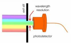
A high resolution (narrow exit slit) in combination with a narrow core input fibre is important to resolve fine spectral detail.
