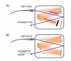
The stray light contribution is measured by blocking the signal beam, see Figure (A). This allows only stray light to exit the monochromator and reach the photodetector.
