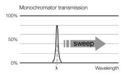
Essentially, the OSA specifications describe the performance of this measuring method. They describe for example; the accuracy, shape, speed and repeatability of the sweeping bandpass filter, but also the accuracy and linearity of the photodetector circuit.
