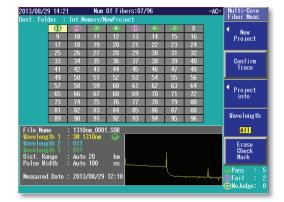
The Multi-Fibre Measurement function automatically performs measurements and data-filling according to a preestablished filename table.
